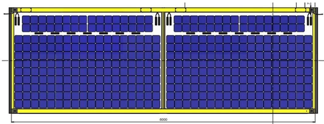
**Figure 3:** The Heijmans modular solar noise barrier panel design. By using a horizontal string on the top part of the modules and vertical strings in the main part, the effects of self-shading are mitigated.
