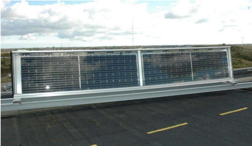
**Figure 2:** A prototype based on the ECN reference design for a bifacial solar noise barrier.
